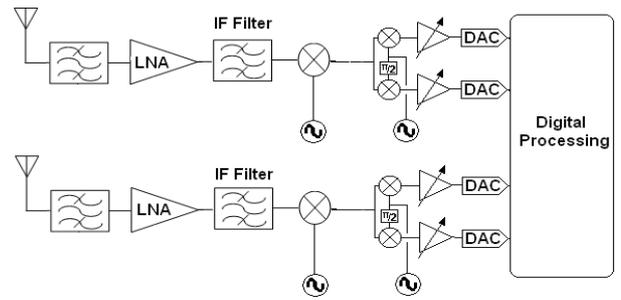
Fig. 3 State of the art of simultaneous reception - Stacked-up heterodyne dedicated front-end architecture.
