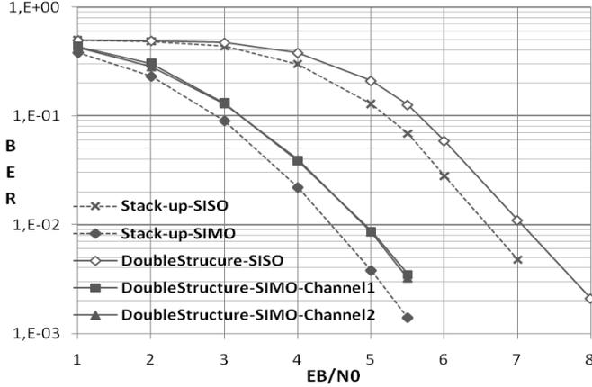
Fig. 7 BER evolution during the simultaneous SIMO reception of a signal composed of two non-overlapping 802.11g channels.
