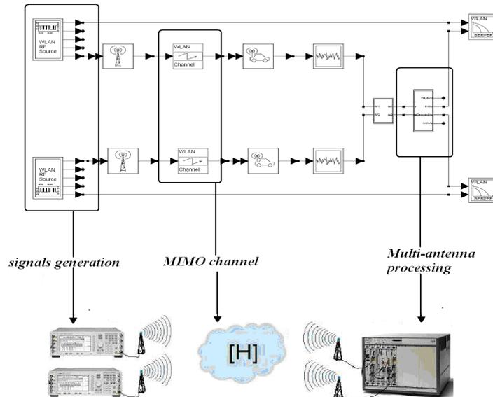
**Figure 1 - The 2x2 MIMO connected solution using the interaction between ADS software and Agilent Technologies equipments. Emitter part, channel propagation and receiver part can be studied and modelled.**
