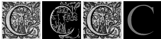
Figure 3: a) Original drop cap image, b) Segmentation of (a) (letter recognized as "S"), c) Opened image (the uppercase is disconnected from the background), d) Segmentation of (c) (letter properly recognized).
