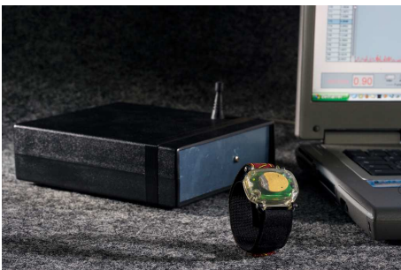
Fig. 2. The Starwatch System : Wireless Sensor, Radio Station and PC
