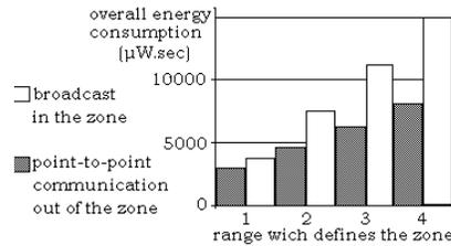
**Figure 4. Energy consumption for broadcast and peer-to-peer communication.**
