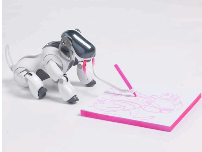
Figure 6: A pen holder extension. ECAL / Meynet Bndicte, Burgisser Olivier, Xavier Rui,Wildi Sbastien et Reymond Simeon Photo : ECAL / Milo Keller
