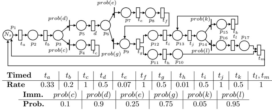
Figure 2: GSPN model of the “order processing” example.
