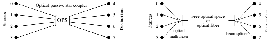
Fig. 2. A degree 4 optical passive star coupler.
