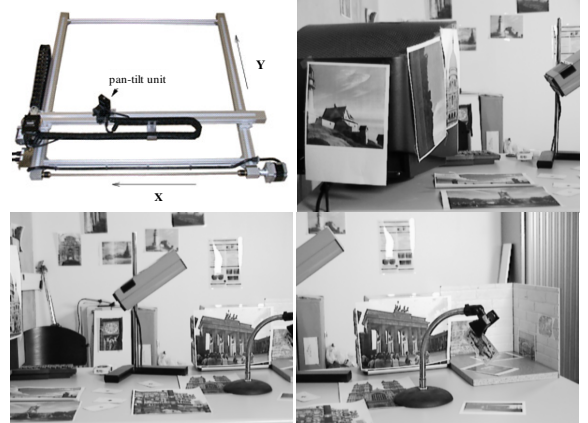
Fig. 1. Top left : The bed used in the experiment to produce the ground truth trajectory. Top right : The initial image for S1 and S2 . Bottom row : The final images of S1 and S2 , respectively.
