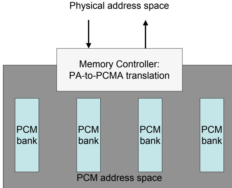
Figure 1: Physical memory address space and PCM memory address space
