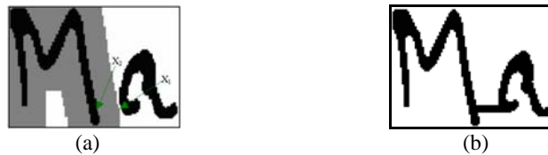
Fig. 3. Joining of isolated characters is shown. (a) A word containing two isolated characters and the grown version of the left component (in gray). (b) Word after joining.
