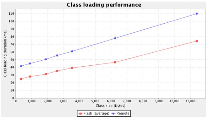
Fig. 6. Class loading time: local vs. remote
