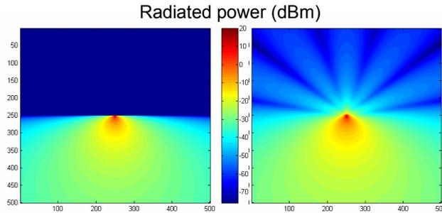
Figure 1. Radiated power in a 500x500 cells free space (5 cm step) for a 20 dBm EIRP
