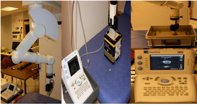
Fig. 7. Experimental setup: (left) medical robot equipped with an US probe transducer - (middle) interaction with an US phantom - (right) interaction with a lamb kidney immersed in a water-filled tank
