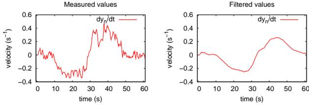
Fig. 9. Measured and estimated velocity of the  $y_n$  visual feature due to the object self-motion.
