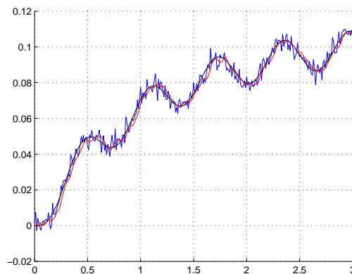
Fig. 1. Noisy output in blue, output without noise in black, and the filtered output using minimal causal estimator in red.
