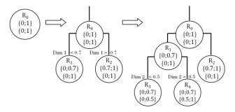
Fig. 3. The sensorimotor space is iteratively and recursively split into subspaces, called "regions". Each region  $R_n$  is responsible for monitoring the evolution of the error rate in the anticipation of consequences of the robot's actions, if the associated contexts are covered by this region.
