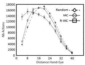
Fig. 6. Histogram of distances repartitions between hand and eye, after 100000 experiments, comparing **Random**, **IAC** and **R-IAC** exploration methods.
