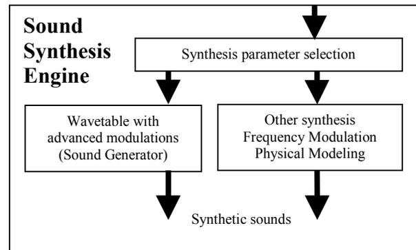
Figure 7: Diagram of the sound synthesis engine.
