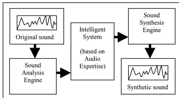
Fig. 2. Conceptual diagram of the intelligent audio system.
