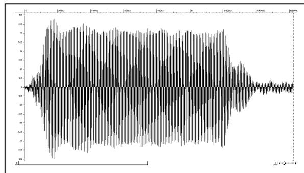
Figure 4: Temporal representation of an organ pipe sound.
