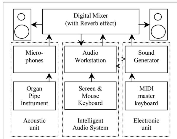
Figure 1: Diagram of the sound design environment.
