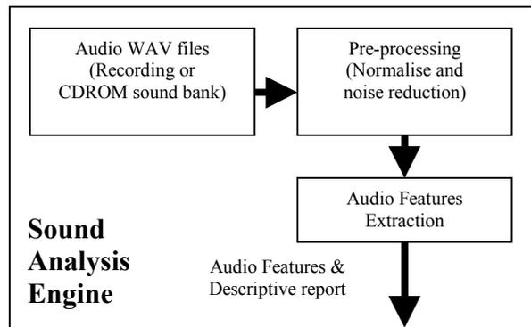
Figure 3: Block diagram of the sound analysis engine.
