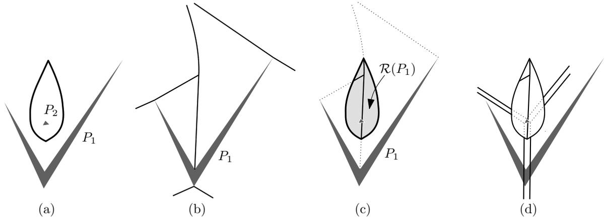
Figure 1: (a) The bisector of two polygons can be a closed curve. (b) The medial axis  $\mathfrak{M}(P_1)$  outside of  $P_1$ . (c) The Voronoi region  $\mathcal{R}(P_1)$ , shown in light gray. (d) The farthest-polygon Voronoi diagram  $\mathfrak{F}(\{P_1, P_2\})$ .
