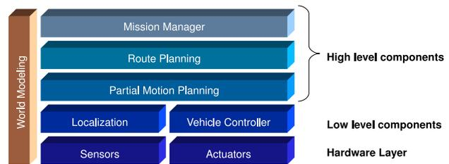
Fig. 1. Overview of the proposed navigation architecture
