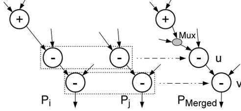
**Figure 6. Multiplexers insertion after pattern merging.**
