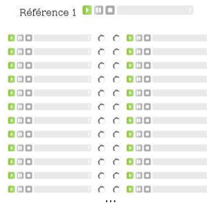
Figure 1. Test 1: for each pair of audio files, the subject selects the one causing more discomfort.
