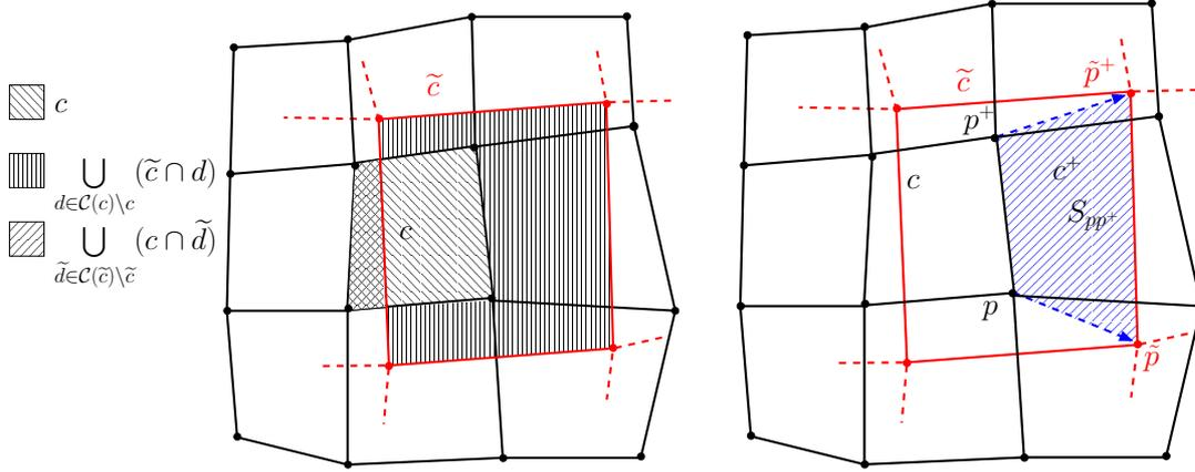
Figure 6: Decomposition of a rezoned cell (left). Swept region resulting from nodes displacement (right).
