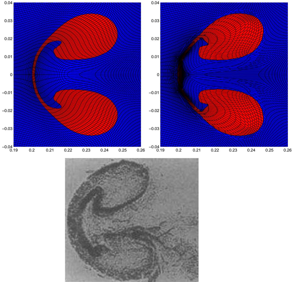
Figure 19: Interaction of a shock wave with an Helium bubble. Zoom on the bubble at  $t_{\text{final}} = 1342.153 \cdot 10^{-6}$  and color map of volume fraction. Cartesian grid on top left, polygonal grid on top right versus Schlieren image from experimental data [20](bottom).
