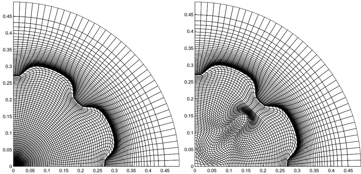
Figure 29: Two-dimensional implosion with perturbed interface. Lagrangian computation with  $a_0 = 2 \cdot 10^{-4}$ . Grids at final time,  $t = 0.3$ , corresponding to the initial polar grid (left) and the initial unstructured (right).
