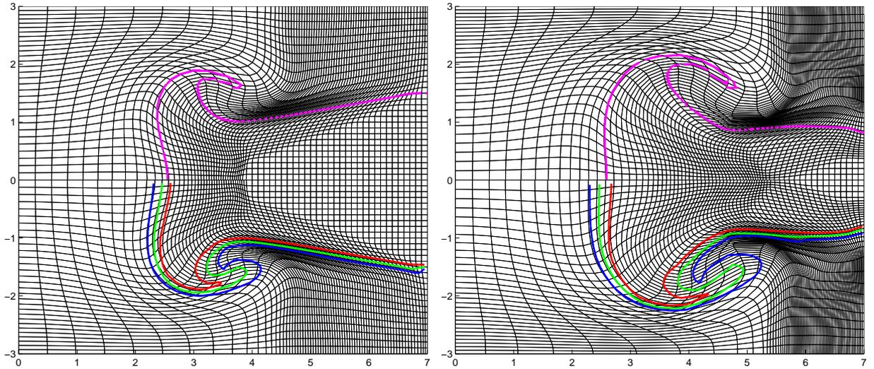
Figure 14: Triple point problem, grid and interface at time  $t = 3.5$  (left) and time  $t = 5$  (right). The top part ( $y > 0$ ) corresponds to the VOF computation and interface is the purple curve. The bottom part ( $y < 0$ ) corresponds to the concentration equations computation, three isolines are plotted:  $C = 0.1$  (blue),  $C = 0.5$  (green) and  $C = 0.9$  (red).
