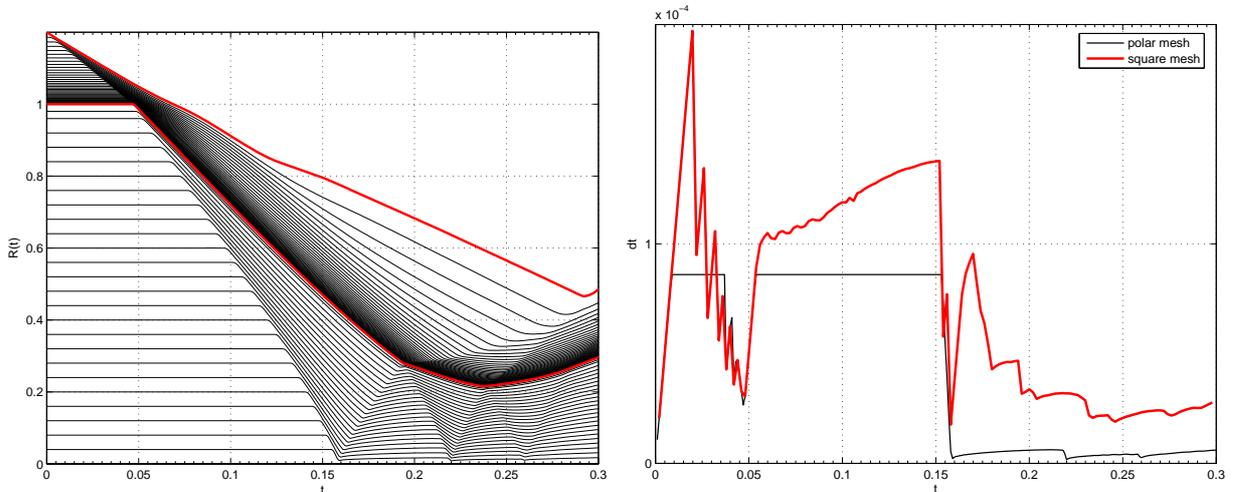
Figure 24:  $t-R$  diagram for the one-dimensional implosion (left). Time step history for the one-dimensional implosion using two-dimensional grids (right). The black curve corresponds to the polar grid while the red one refers to the unstructured grid.
