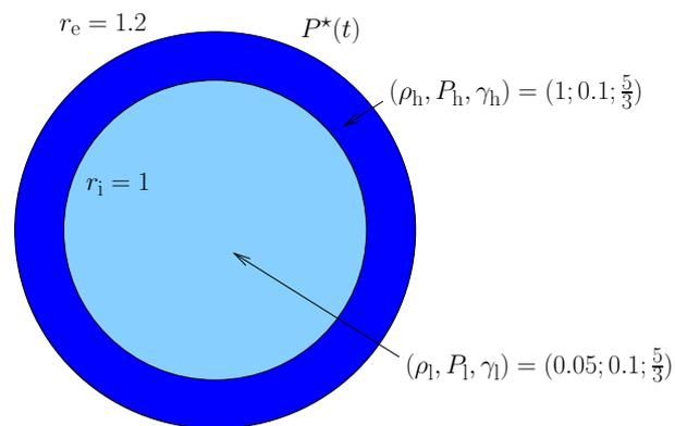
Figure 23: One-dimensional implosion. Initial geometry and data.
