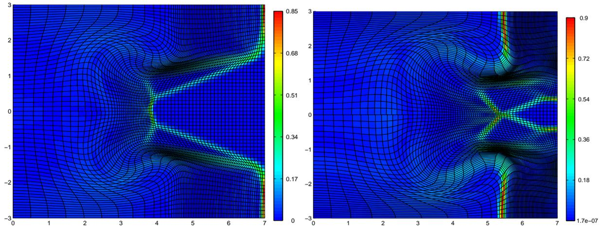
Figure 15: Triple point problem, map of  $\omega_p$  at time  $t = 3.5$  (left) and time  $t = 5$  (right). The top part ( $y > 0$ ) corresponds to the VOF computation and the bottom part ( $y < 0$ ) corresponds to the concentration equations computation.
