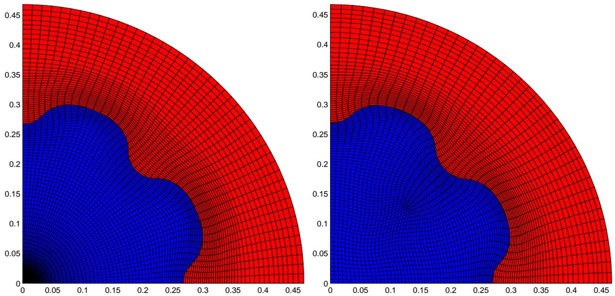
Figure 31: Two-dimensional implosion with perturbed interface  $a_0 = 2 \cdot 10^{-4}$ . Grids and interfaces at the final time,  $t = 0.3$ , corresponding to the initial polar grid (left) and the initial unstructured grid (right).
