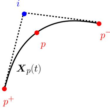
Figure 4: Boundary node treatment: notations for the Bezier curve.  $p^-$ ,  $p$  and  $p^+$  are vertices located on the boundary. The second-order interpolation Bezier curve,  $\mathbf{X}_p(t)$  is plotted in black.
