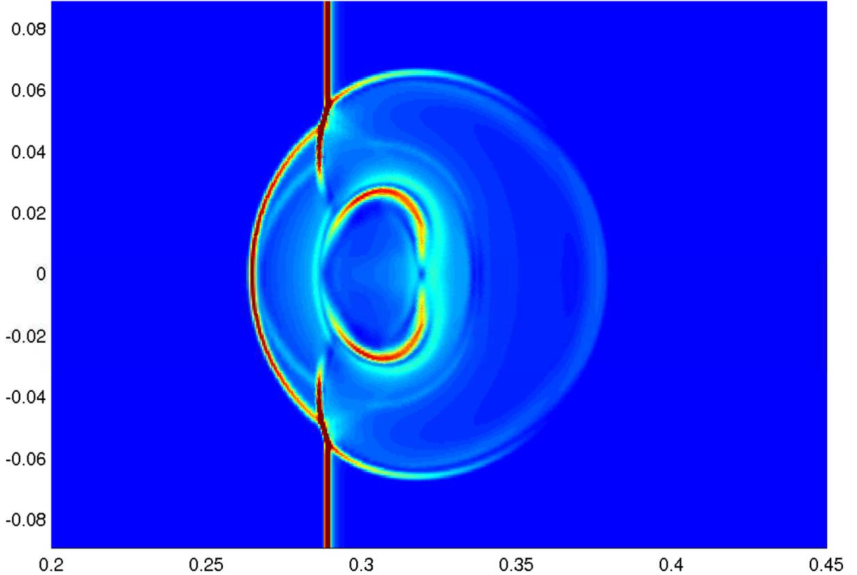
Figure 21: Interaction of a shock wave with an Helium bubble. Map of  $\omega_p$  parameter in the vicinity of the bubble for a twice finer Cartesian grid at  $t = 800 \cdot 10^{-6}$ . The red color indicates the maximum value, i.e. it shows the regions where the maximum deformation occurs.
