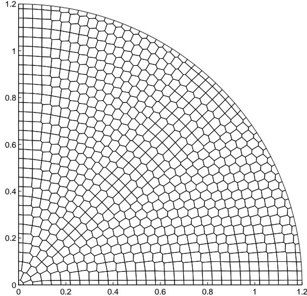
Figure 11: Initial unstructured polygonal grid for the Sedov problem.
