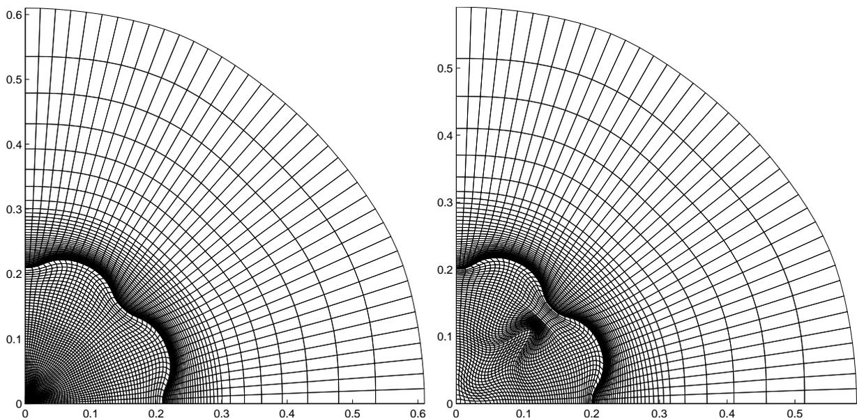
Figure 30: Two-dimensional implosion with perturbed interface. Lagrangian computation with  $a_0 = 10^{-3}$ . Grids at failure time,  $t_{\text{fail}} = 0.24$ , corresponding to the initial polar grid (left) and the initial unstructured (right).
