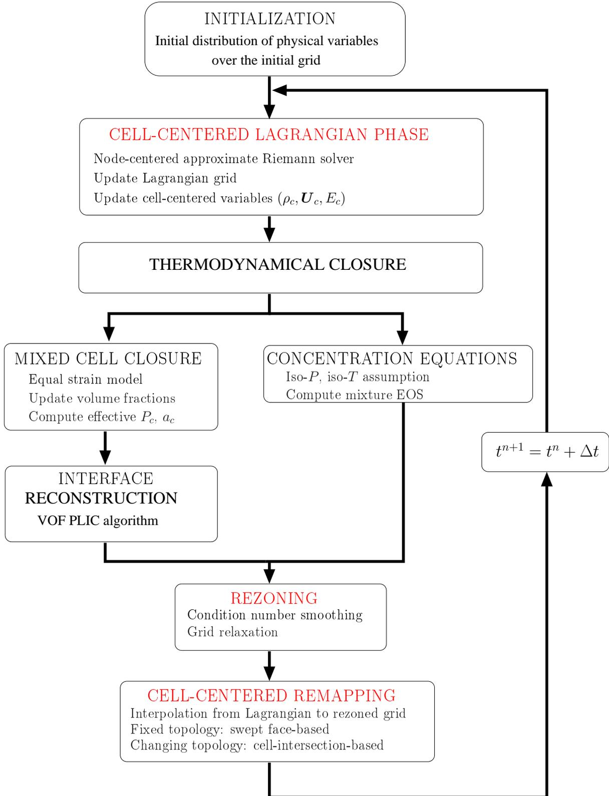
Figure 1: Flowchart of the multi-material ALE algorithm.
