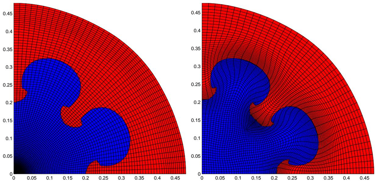
Figure 32: Two-dimensional implosion with perturbed interface  $a_0 = 10^{-3}$ . Grids and interfaces at the final time,  $t = 0.3$ , corresponding to the initial polar grid (left) and the initial unstructured grid (right).
