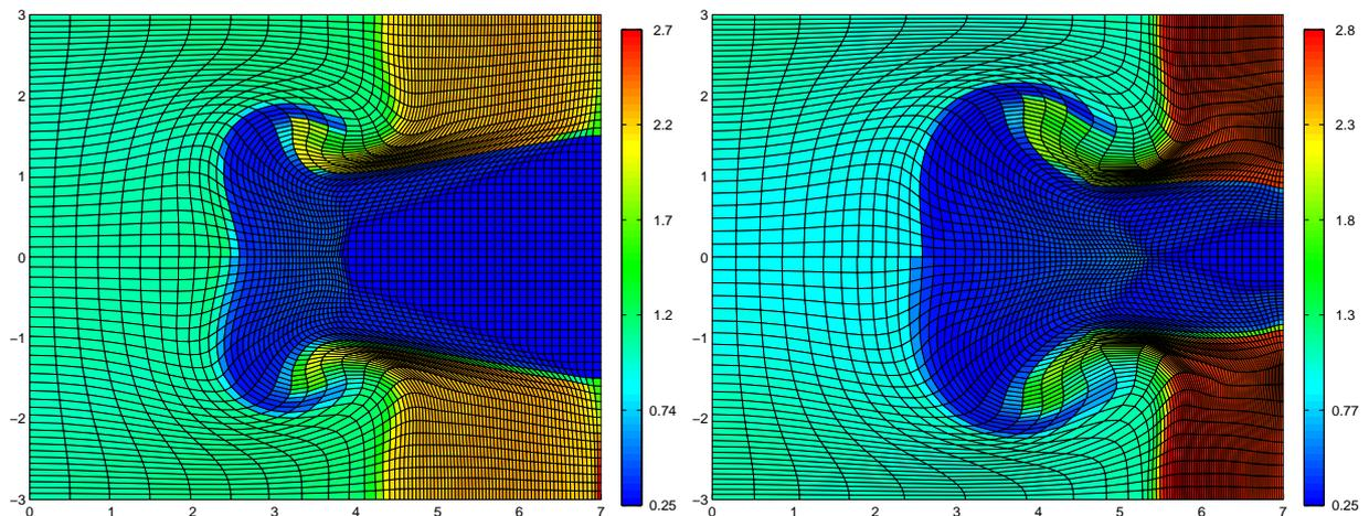
Figure 16: Triple point problem, map of specific internal energy at time  $t = 3.5$  (left) and time  $t = 5$  (right). The top part ( $y > 0$ ) corresponds to the VOF computation and the bottom part ( $y < 0$ ) corresponds to the computation done using concentration equations.
