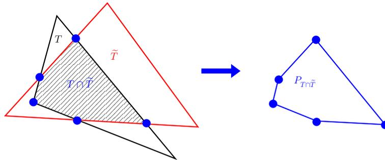
Figure 8: Sub-polygon that results from triangle-triangle intersection
