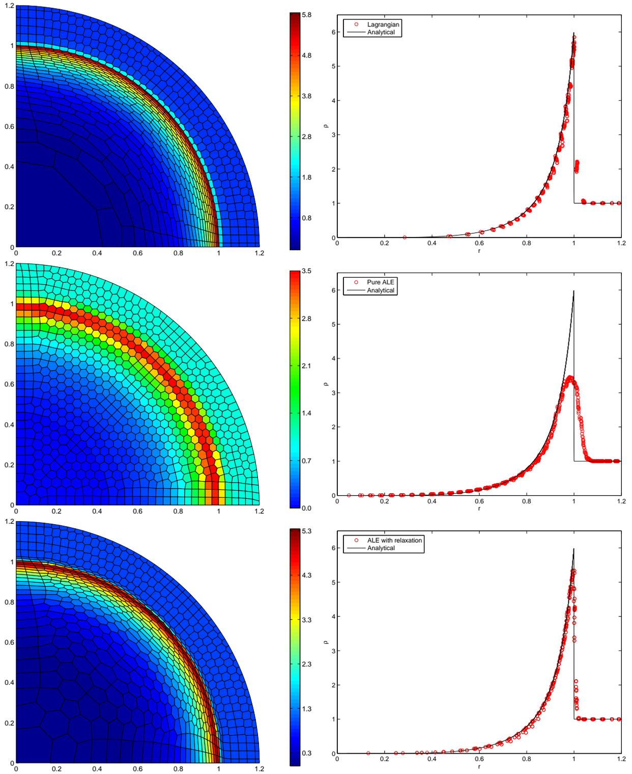
Figure 12: Sedov problem at final time  $t = 1$ . From bottom to top, ALE computation with relaxation procedure, ALE computation with pure rezoning ( $\omega_p = 1$ ) and Lagrangian computation. Left column: density map and grid, right column: density as a function of the radius of cell centers versus analytical solution.
