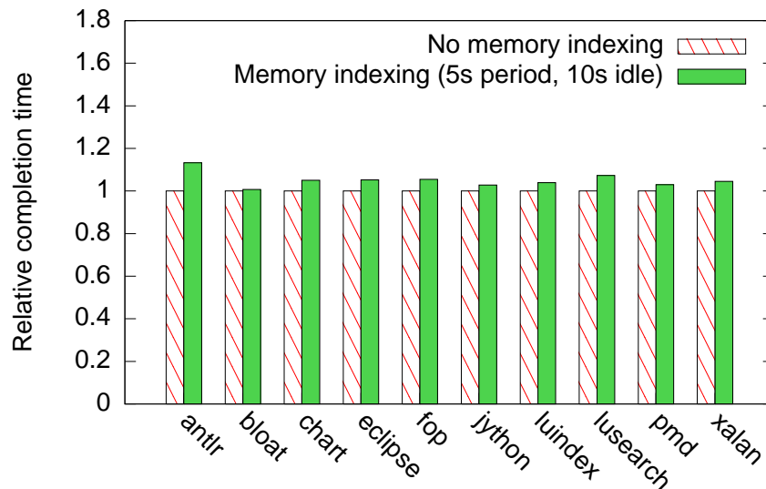
Figure 8: Relative performance of Dacapo benchmarks with periodic memory indexing
