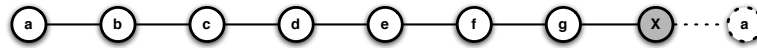
Figure 10: Link Spoofing: The malicious router X advertises a spoofed link to router a in its TC messages, thus all routers will record the links X-a and b-a .
