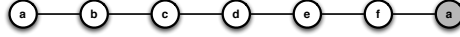
Figure 16: Identity Spoofing: the gray malicious router spoofs the identity of router a .
