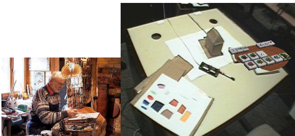
Figure 2: A real studio (left image) and our virtual studio (right image). In the right image, we see a tool palette to the right, a tracked pencil in the center, a scratch area into the left, and a physical house model on the working surface towards the top.
