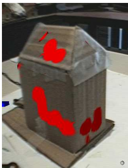
Figure 4: Painting with only geometry information. Paint is simply blended with the current color on the transparent texture of the object. Note that there is no mix with the appearance of the real object.
