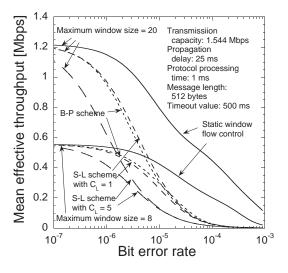
(b) In the case of multiple-NACK selective ARQ error recovery Fig. 2 Comparisons of performance of B-P and S-L schemes.
