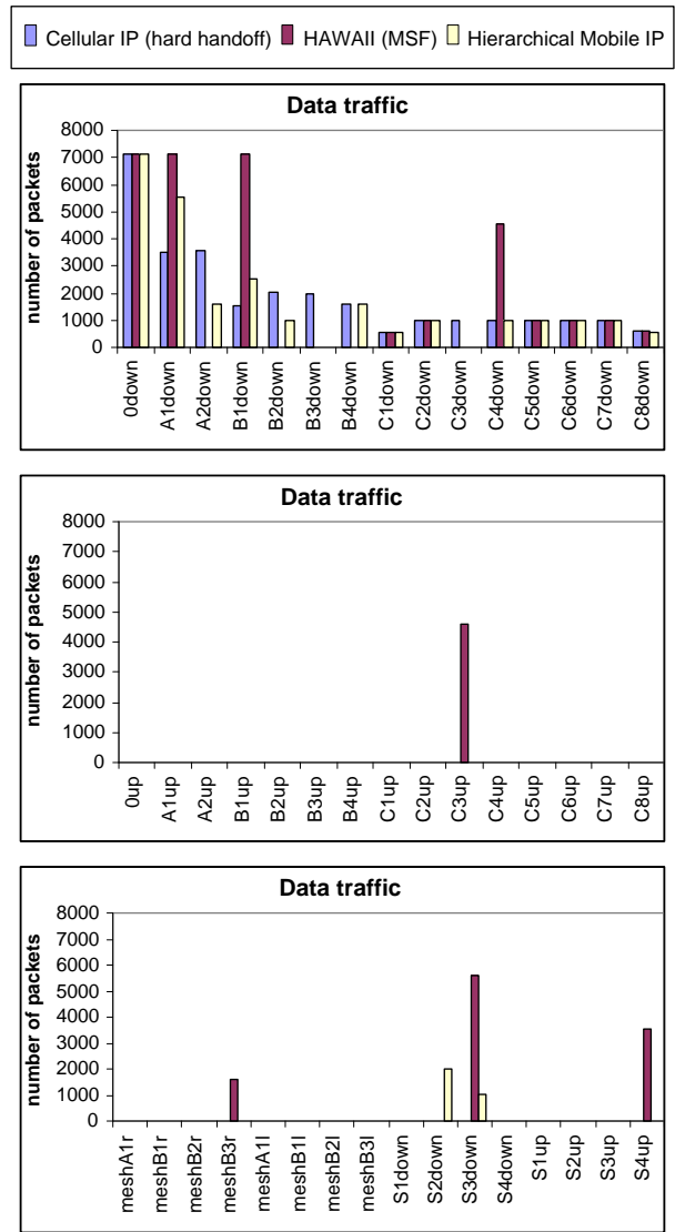
Fig. 7. Average number of data packets on the links of the access network during 1 simulation.
