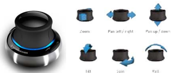
Figure 3. The SpaceNavigator and its degrees of freedom.
