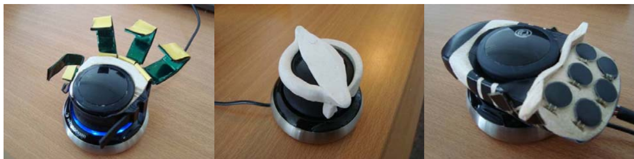
(a) The first shape based on the one of the V2 prototype. (b) The second shape based on the one of the SpaceNavigator. (c) The third shape based on the one of a computer mouse.
