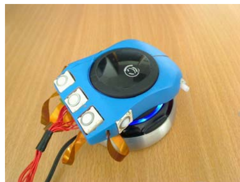
(b) The V5 prototype integrates only trackballs.
