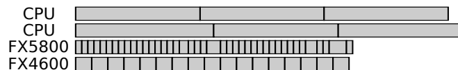
Figure 9: A pathological case: Gantt diagram of a blocked matrix multiplication with a greedy strategy.
