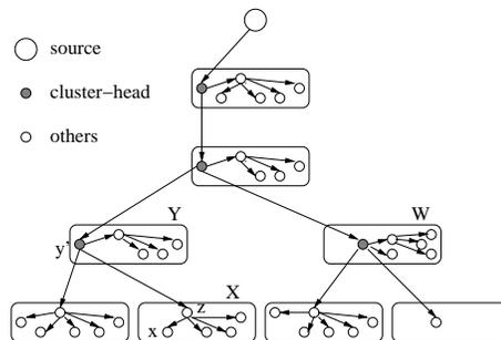
Figure 2: Multicasting inside a cluster tree of PrefixStream.
