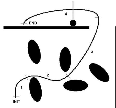
Figure 3: A path made of 4 Bezier curves
