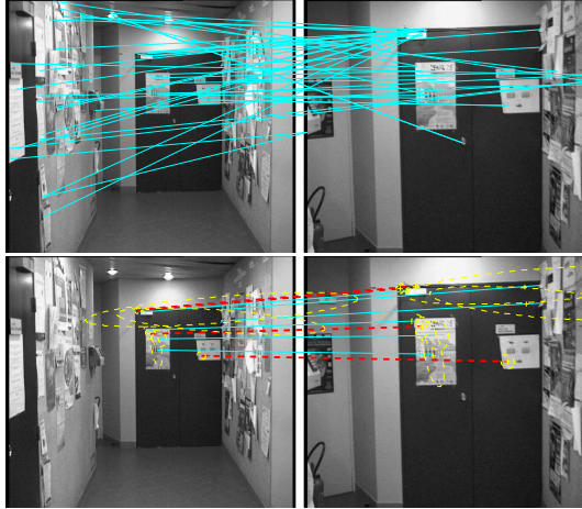
Figure 1. Top: 44 SIFT correspondences. Many outliers can be seen. Bottom: 10 inliers are retrieved with our algorithm. Please zoom in on the pdf file.
