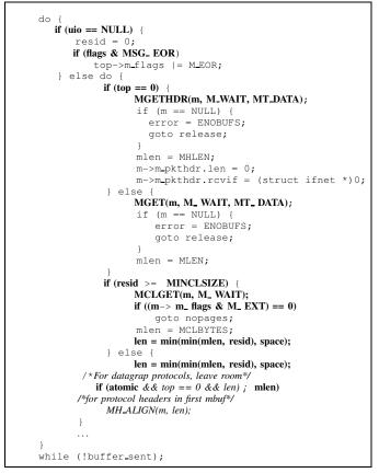
Fig. 2. Fast-path of the UDP send operation in BSD
