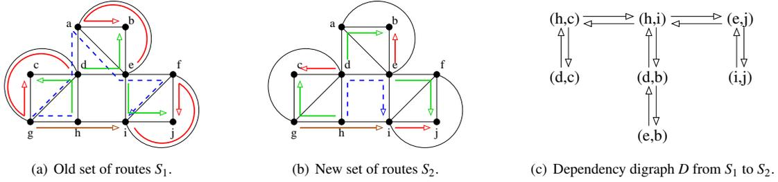
FIG. 1: Instance of the reconfiguration problem consisting of a network with 10 nodes, symmetric arcs, and 8 connections  $(h,i)$ ,  $(h,c)$ ,  $(d,c)$ ,  $(d,b)$ ,  $(e,b)$ ,  $(e,j)$ ,  $(i,j)$ ,  $(g,i)$  to be reestablished.
