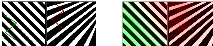
Fig. 1. Failure of standard colorization algorithms in presence of texture. Left: manual initialization; right: result of Levin et al. 's approach. In spite of the general efficiency of their simple method (based on the mean and standard deviation of local intensity neighborhoods), texture remains difficult to deal with. Hence the need of texture descriptors and of learning edges from color examples.
