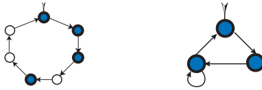
The language O \subset O^* over the one-letter alphabet \{0\} is equivalently defined by: O = \{0^n : (n \bmod 7) \in \{0, 1, 2, 4\}\} . The graph of its minimal deterministic automaton \text{MDA}(O) is drawn above to the left. The graph of its minimal nondeterministic Xor automaton \text{MXA}(O) is to the right.
