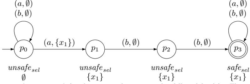
Figure 3: Automaton  $A$  for the query selecting  $a$ -nodes followed by  $b$ - $b$ . There are two reachable unsafe states of type  $\{x_1\} = \mathcal{V}_1$ ,  $p_1$  and  $p_2$ . The restriction of  $A$  to these two states is acyclic, so the selection delay of  $Q_A$  is bounded. It is bounded by 2, since the longest path in this part of the automaton has 2 nodes.
