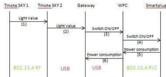
Figure 13: IEEE 802.15.4 frames exchange diagramm
