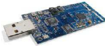
Figure 7: Tmote SKY platform from Crossbow
