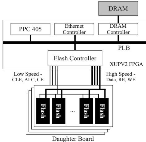
Figure 1: The overall architecture of BlueSSD.
