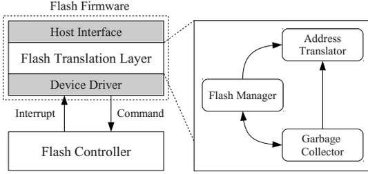
Figure 2: The overall structure of the flash firmware.
