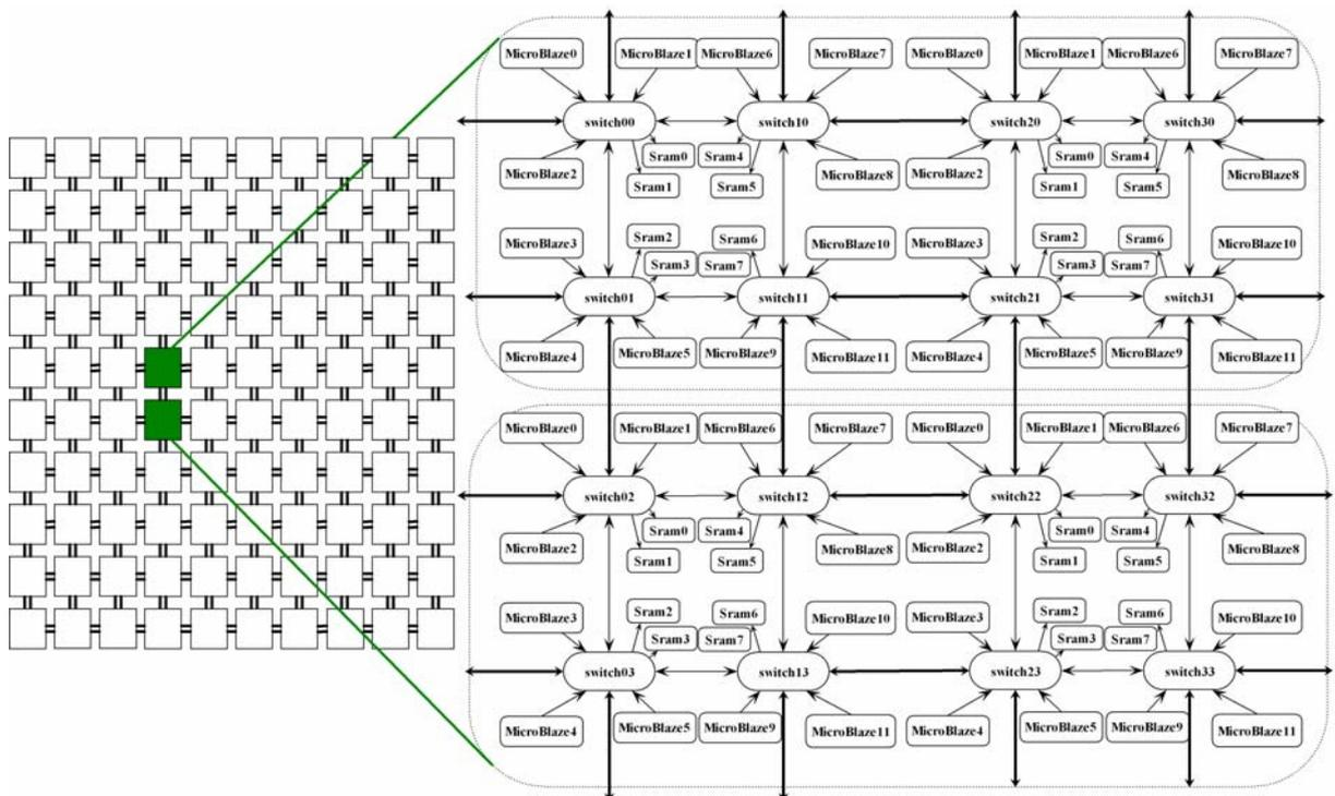
Figure 2 Extension to 2400-cores NOC based MPSOC.
