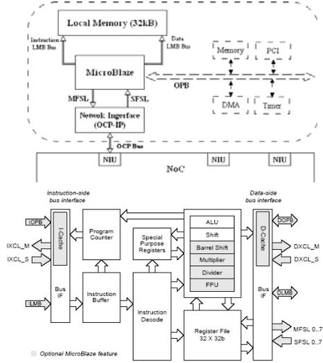
Figure 3 (a) Processor Tile (b) MicroBlaze core block diagram
