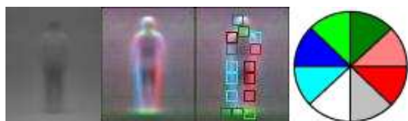
Figure 3. Mean human image with corresponding edge magnitudes and the 15 most dominant cells.
