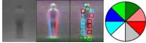
Figure 1. Mean human image with corresponding edge magnitudes and the 15 most dominant cells. From the left: the first image shows the mean human image calculated over all positive samples in the database; the second image shows the corresponding mean edge magnitude response; the third image shows this later image superposed with the 15 most dominant cells of size 8 \times 8 pixels.
