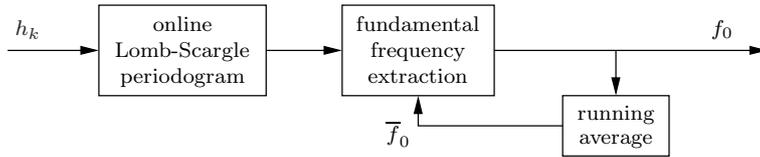
Figure 2: The RTT estimation process: after the update of the spectrum estimation, the fundamental frequency  $f_0$  is extracted; the RTT estimation is the inverse of  $f_0$ .
