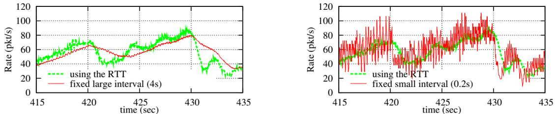
Figure 1: Rate estimate using the estimated RTT, compared with the same using two fixed averaging intervals: large interval (left) and small interval (right).
