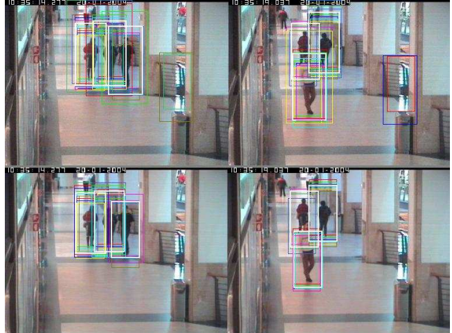
Figure 3. Examples of filtered detected person candidates in a Caviar sequence
