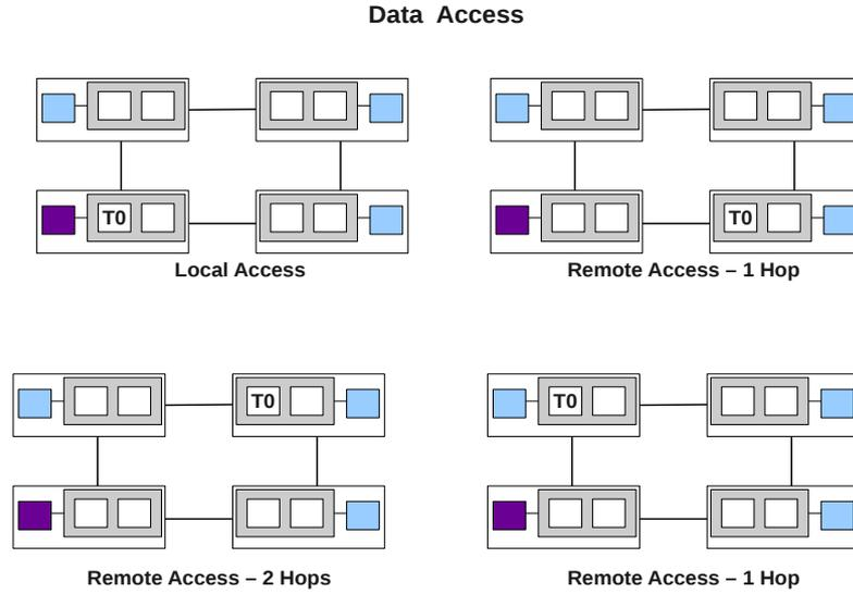
Figure 7: Local and Remote Data Access Performed by Thread T0.
