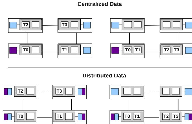
Figure 8: Centralized and Distributed Data and Threads Placement.
