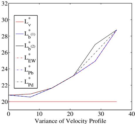
Fig. 4. Optimal cell size versus variance of the velocity.
