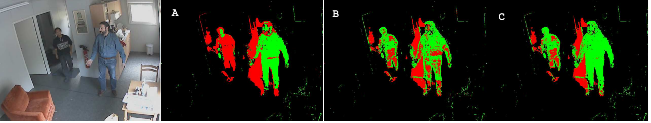
Figure 3. Shadow detection results of the algorithm using only chromaticity constraint (image A), of the algorithm using only texture constraint (image B) and of the combination of these two algorithms (image C). Chromaticity and texture complement each other to have a better result.
